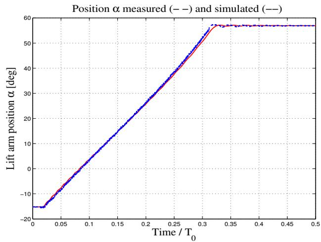
Fig. 9. Lift arm angular position  $\alpha$  measured (dashed) and simulated (solid) for an hitch lift with light load.
