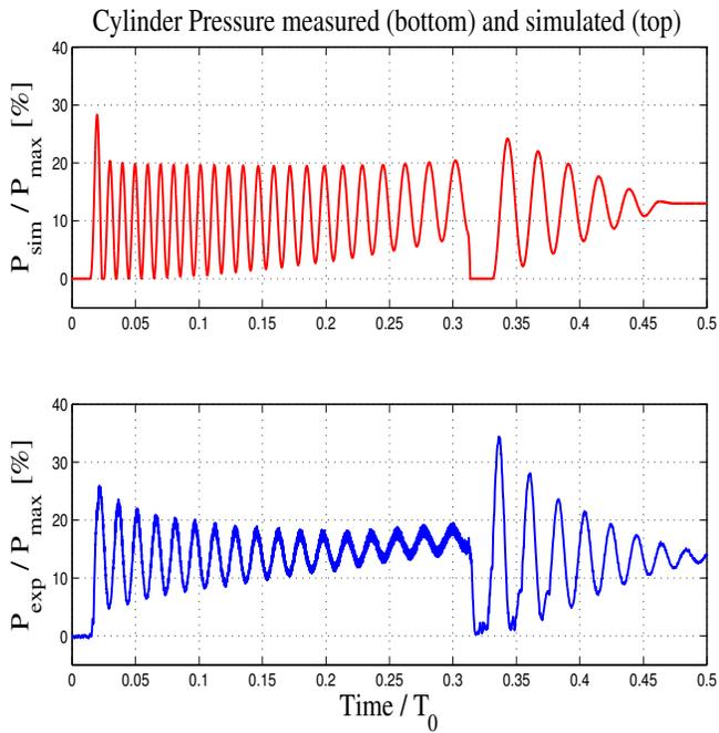
Fig. 8. Cylinder pressure  $P$  measured (bottom) and simulated (top) for an hitch lift with light load.
