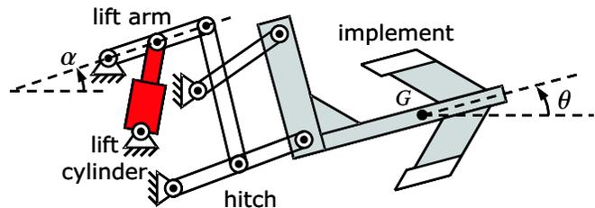
Fig. 1. Three point hitch for a farm tractor.
