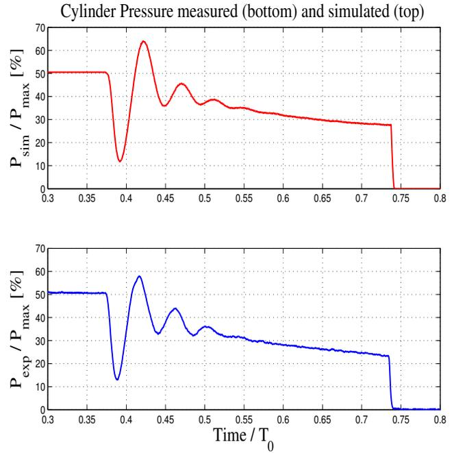
Fig. 6. Cylinder pressure  $P$  measured (bottom) and simulated (top) for an hitch fall with heavy load.
