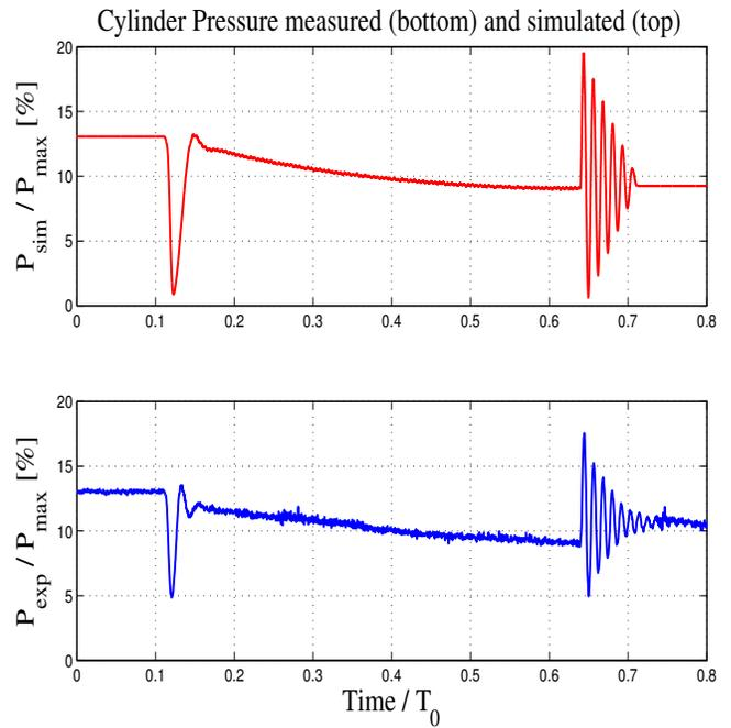
Fig. 10. Cylinder pressure  $P$  measured (bottom) and simulated (top) for an hitch fall with light load.
