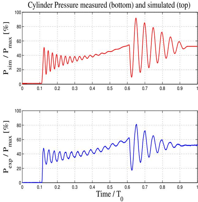
Fig. 4. Cylinder pressure  $P$  measured (bottom) and simulated (top) for an hitch lift with heavy load.
