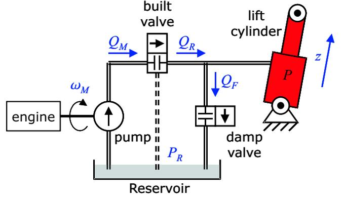
Fig. 2. Schematic of the standard electro-hydraulic components of a three point hitch.
