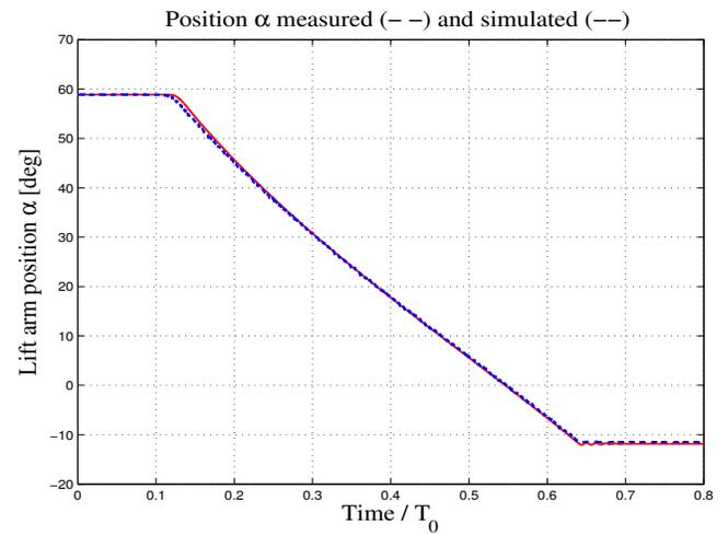
Fig. 11. Lift arm angular position  $\alpha$  measured (dashed) and simulated (solid) for an hitch fall with light load.
