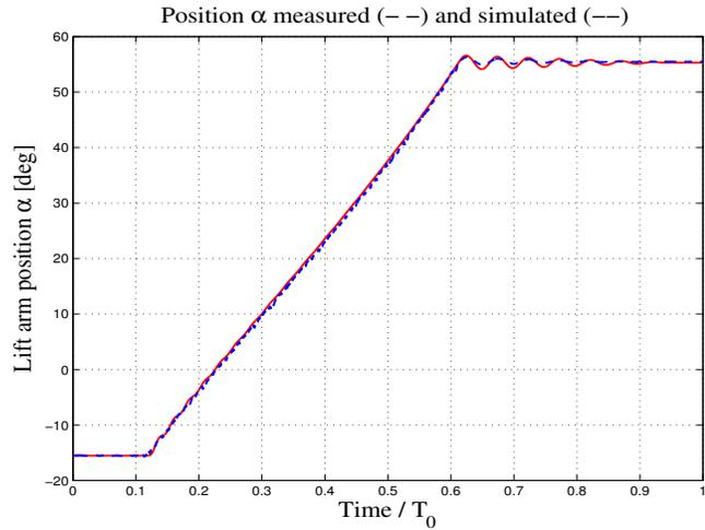
Fig. 5. Lift arm angular position  $\alpha$  measured (dashed) and simulated (solid) for an hitch lift with heavy load.
