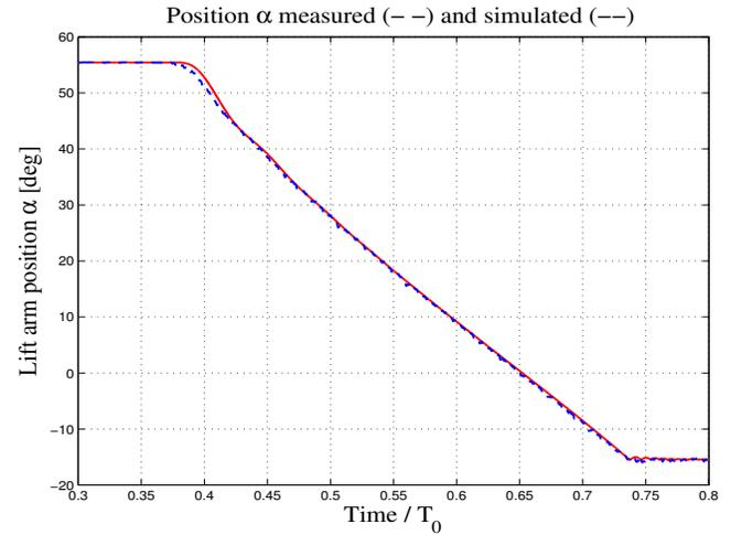
Fig. 7. Lift arm angular position  $\alpha$  measured (dashed) and simulated (solid) for an hitch fall with heavy load.
