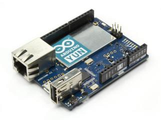
Atheros AR9331 processor, running Linux and the OpenWrt wireless stack
