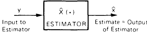
Fig. 2.3-1 The estimator is a function, or a device for assigning a number, given a measurement.
