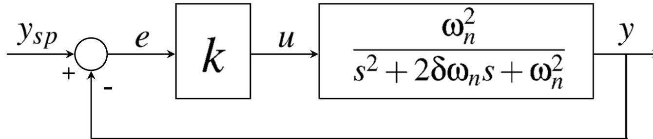
$$F(s) = \frac{\frac{k}{1+k} \bar{\omega}_n^2}{s^2 + 2\bar{\delta} \bar{\omega}_n s + \bar{\omega}_n^2} \quad \bar{\delta} = \frac{\delta}{\sqrt{1+k}}$$
