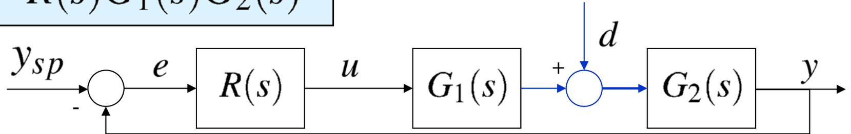
$$Y = \frac{L(s)}{1 + L(s)} Y_{sp} + \frac{G_2(s)}{1 + L(s)} D \quad \Rightarrow \quad Y = F(s) Y_{sp} + G_2(s) S(s) D$$
