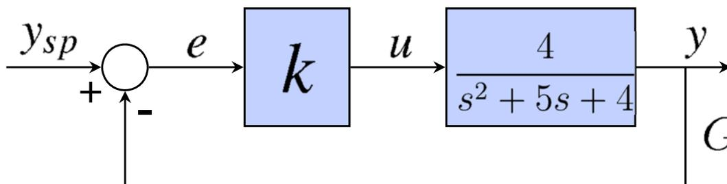
$$G_{c.l.}(s) = \frac{\frac{k}{1+k}\bar{\omega}_n^2}{s^2 + 2\bar{\delta}\bar{\omega}_n s + \bar{\omega}_n^2}$$
