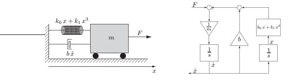
where u = F represents the input of the system,  $y = \dot{x}$  is the output and the parameters'values are m = 1 Kg,  $k_0 = 0.5$  N/m  $k_1 = 0.25$  N/m<sup>3</sup>, b = 0.75 M s/m:
